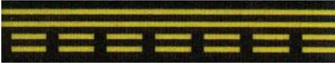
Runway Holding Position Marking
