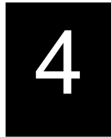
Runway Distance Remaining (RDR) Sign
