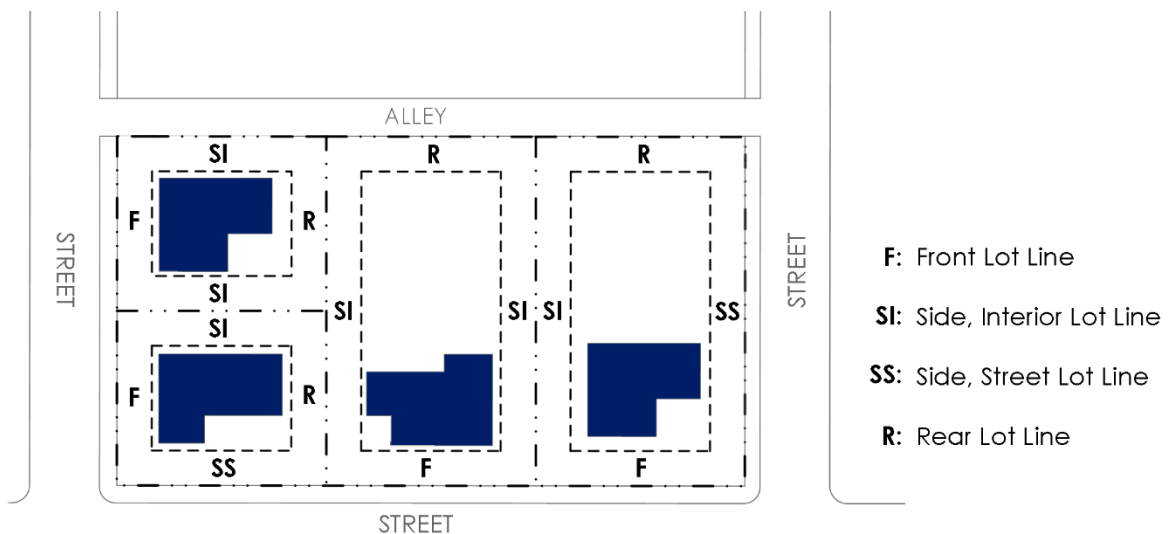
Fig. 20-19-C. Lot Lines on Interior and Corner Lots
